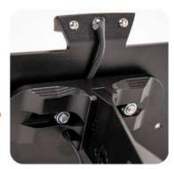
4) a/ Place the light wire between the two holes in the plate holder.
