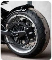
6) a/ Place the plate holder on the left side of the motorbike using the original rear wheel axle.
